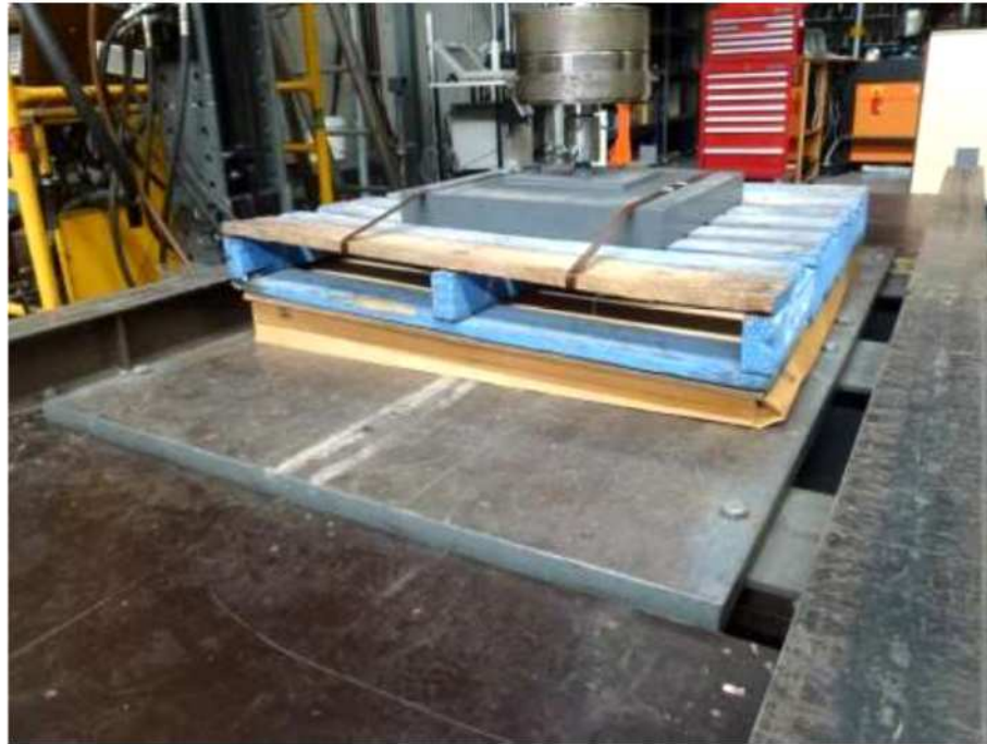
FIG.3 150MM SUPAVOID LOAD TEST AT FAILURE
